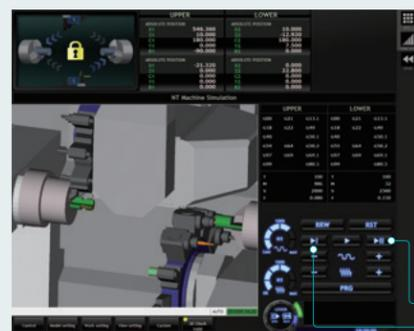
Simulation is performed while checking the remaining movement amount and modal information.
