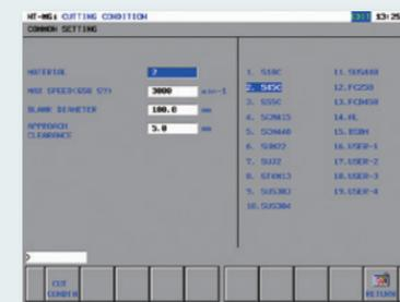
By selecting the material, cutting conditions B are automatically input.
