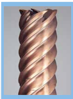
Wear pattern d 8 mm after 58 min operating time
